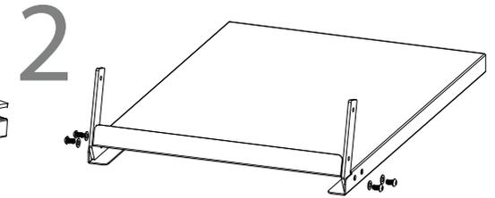
Mount the L brackets on the base. The short side is fixed to the base, the long side is fixed to the main body in the next step.
