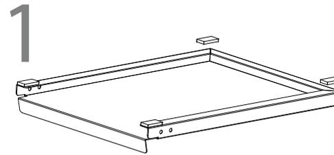
Attach the included felt pads to the base.
