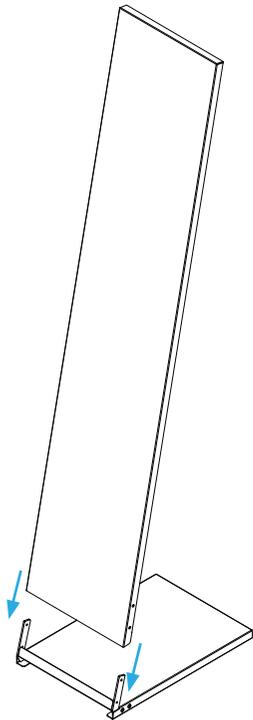
Place the main body on the L brackets. The easiest way to do this is to place the base on the floor and attach the main body from above.
