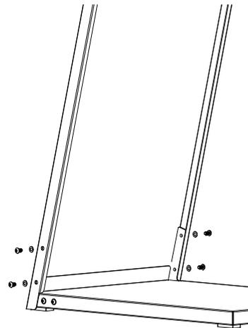
Use the screws and washers to tighten the main body onto the L brackets
